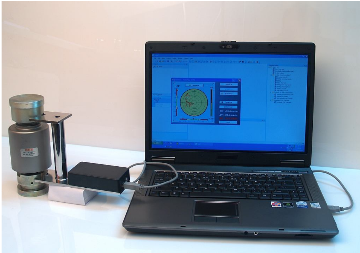
The Electronic Level - cooperation with the PC via USB port
